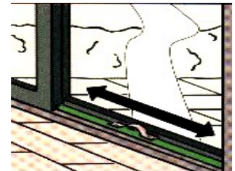
Lat of stok in geleiderrail
